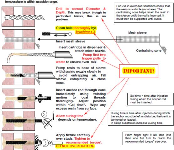
SAMPLE METHOD STATEMENT - RESIN INJECTION ANCHORS - In hollow materials
