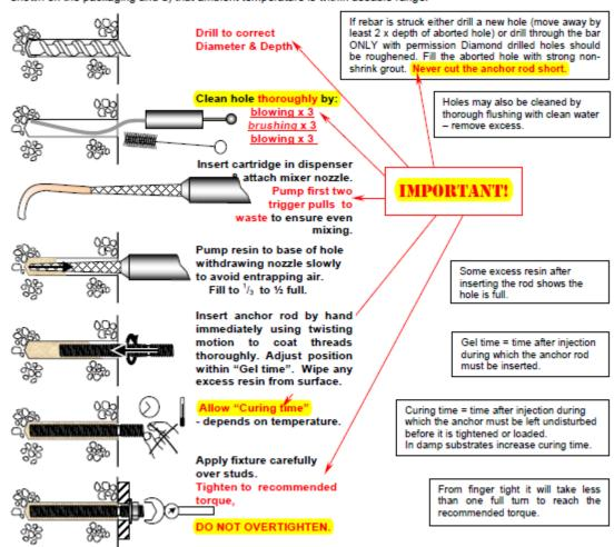
SAMPLE METHOD STATEMENT - RESIN INJECTION ANCHORS - In Concrete
